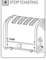
The 'timer' will dick off to 'O' position. To cancel toasting manually rotate the 'timer' to 'O'. If neon light remains illuminated after use immediately unplug the toaster & call service centre.
